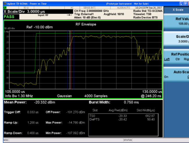
Figure 2-12 Power vs. Time - Zoom in (Ref Value = 105 \mu s, Scale/Div = 3 \mu s)
